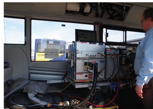
Emissions comparison of CNG and diesel powered buses using a PEMS instrument
